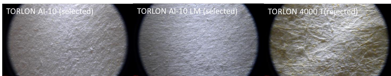
Fig.4: Optical microscope images (same magnification) of selected Torlon AI-10 (left) and Torlon AI-10 LM (centre) and rejected Torlon 4000 T (right)
