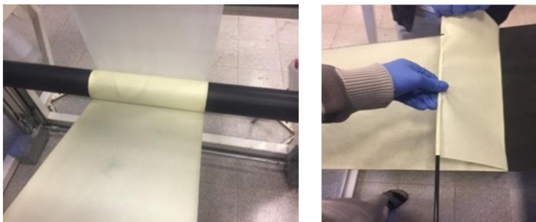
Fig.7: Manufacturing of Torlon PAI force-spun roll (left) and peeling off of Torlon film (pale yellow) from textile support (black) using the discharge rod (right).
